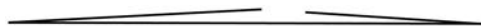
Figure 10.11 There Is No Way to Make a Triangle With Three Lengths of 7, 13, and 5 Centimeters
